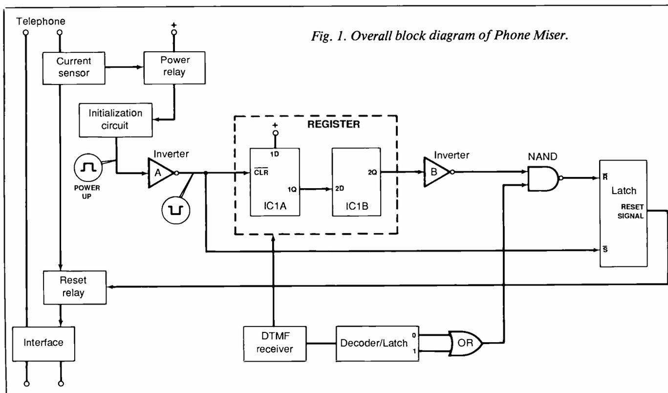
Fig. 1. Overall block diagram of Phone Miser.
