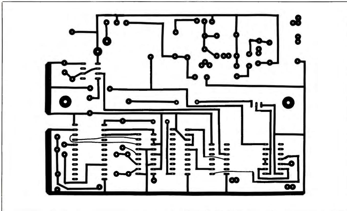
Fig. 5. Actual-size etching-and-drilling guide for printed-circuit board.
